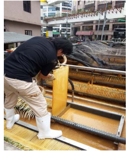
PVDF element-without sludge caking !
